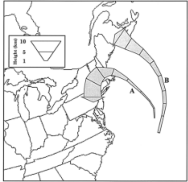
FIG. 11. Representative 24-h forward trajectories initialized in the warm sector boundary layer at 1200 UTC 31 March 1997 from the UW-NMS. Height of air parcels indicated by width of trajectory arrow according to legend. Tick marks identify 3-hourly positions of air parcels. See text for discussion of A and B.
