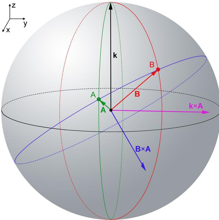
**Fig. 8** A geometric figure to aid the description of how great-circle distance and initial bearing is calculated, which is used in plotting Figs. 4, 5, 6 and 7
